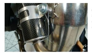
guide the safety wire on one side around the stud of the bracket mount and on the other side around the end tube as shown. Care for a tight fit and make wire as short as possible
